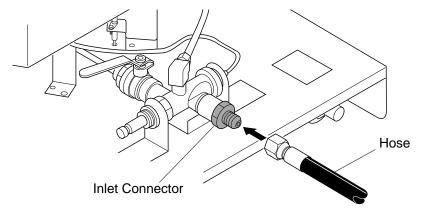
Figure 3 - Hose and Inlet Connector
